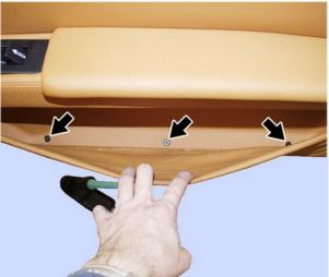
• Remove the three plugs (2) which secure the internal weather strip to the door frame.
